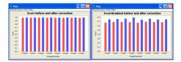
Crosscorrelation of the overlapping areas of the calibration images before (red) and after (blue) the correction is applied. The gradient is shown because it concentrates on edges in the image and these are the image element most people want to match, e.g. for later stitching.
