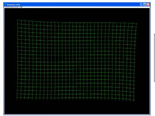
A grid transformed according to the estimated distortion. This is useful to see which kind of deformation is present in the image.
